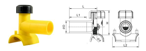
Kimplas Electrofusion Tapping Tees, manufactured in PE100 (Black) grade are SDR 11 rated (PN 16). Kimplas Electrofusion Tapping Tees are suitable for Tapping House Service Connections on MDPE 80 and PE 100 pipes, both in straight as well as coil form.
